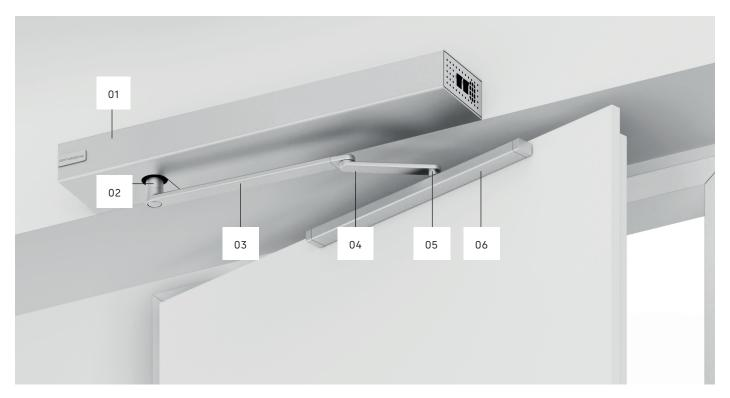
The ED door operator can be mounted on either the hinge or the opposite hinge side, depending on the requirements. Depending on the reveal depth and position in relation to the door leaf, a customized solution is created from a Slide Channel Set or ED standard arm, spindle extension and lever bolt variant. The following slide channel sets can be used in combination with an ED 100 or ED 250 on doors on the hinge side (pull version):
